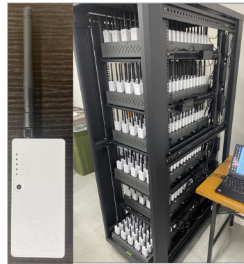
Figure 4: Implemented transmitter Left 1 transmitter enlarged, right 500 transmitters
