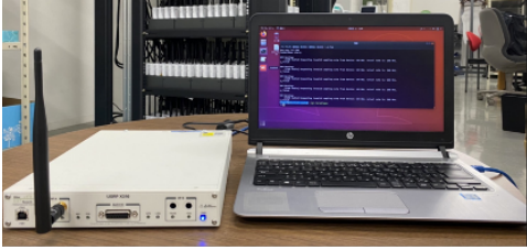
Figure 6: Implemented receiver Left USRPX310, right PC
