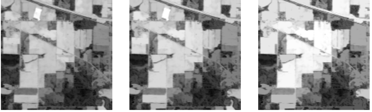
Fig. 1: Morphological opening profile built on the first PC of hyperspectral image. The scale of circular SE varies from 2 to 6, with step size increment of 2. As the size of the SE increases in openings, more small bright objects disappear in the dark background.
