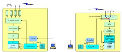
Figure 1: Measurement systems (left: Transmitter, right: Receiver)
