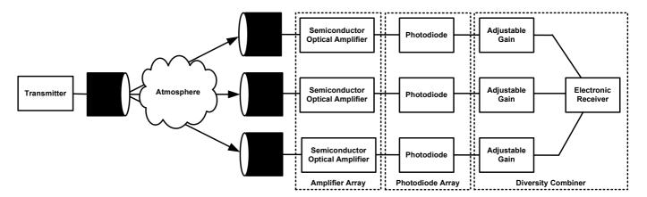
Fig. 1. Optically pre-amplified system with diversity
