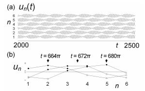
Fig. 3. Traveling phase wave in a ring of six oscillators.
