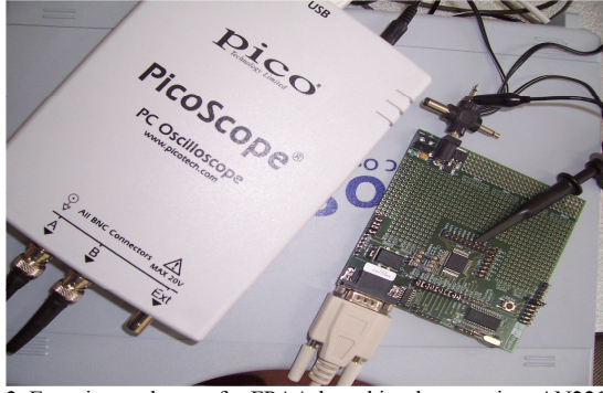
Fig.2. Experimental setup for FPAA-based implementation. AN221E04 type FPAA produced by Anadigm [3] has been used in this setup.
