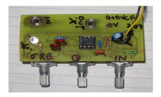
Figure 3: Physical Implementation of the Chaotic Circuit.
