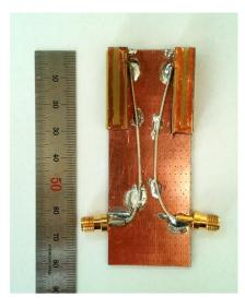
Figure 2: Photograph of fabricated MIMO antenna.
