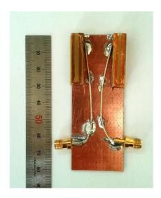
Figure 2: Photograph of fabricated MIMO antenna.
