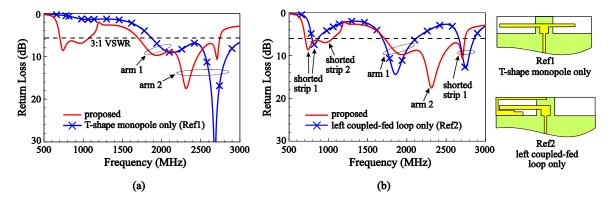
Fig. 3: Simulated return loss for (a) the proposed antenna and the case with the T-shape monopole only (Ref1), and (b) the proposed antenna and the case with the coupled-fed loop on the left-hand side (arm 1 and shorted strip 1) only (Ref2).
