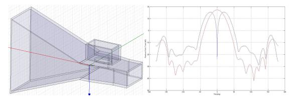
Figure 2: Cross-section of multimode monopulse feed horn and simulated radiation characteristics.
