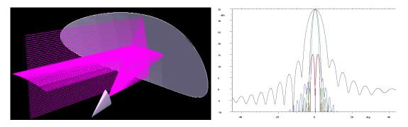
Figure 1: Parabolic reflector antenna and simulated radiation characteristics.
