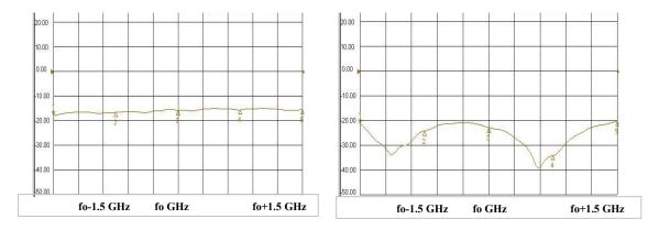
Figure 4: Measured return loss of sum and difference ports of parabolic reflector antenna.
