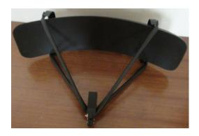
Figure 3: Realized reflector assembled with multimode feed horn.
