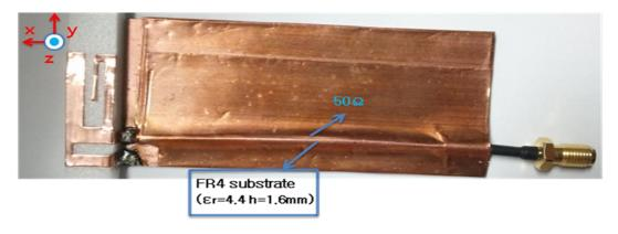
Figure 1: Photo of the implemented antenna.
