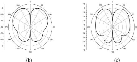
Figure 4: Simulated *y*-*z* plane radiation patterns of Button Antenna (a) 3.5GHz; (b) 6GHz; (c) 9GHz.
