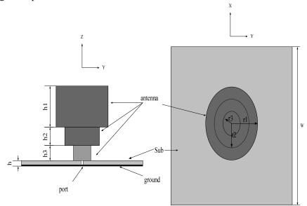
Figure 1: Dimensions of the UWB button.
