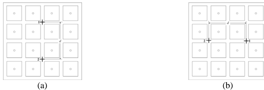
Figure 3: Feed Center of Radiator (a) 1 \times 2 Array Elements and (b) 2 \times 1 Array Elements.
