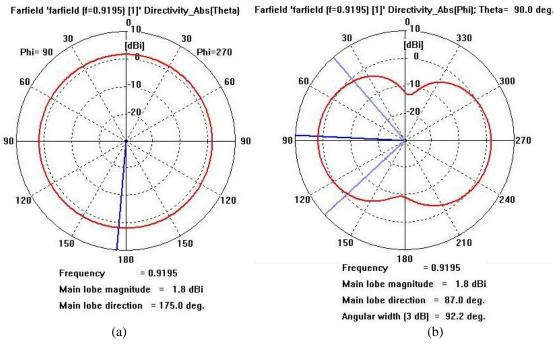
Figure 4. Radiation pattern for (a) H-plane (b) E-plane
