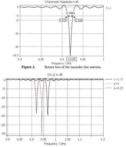
Figure 3. Resonant frequencies for the variation of the spacing between the pitch
