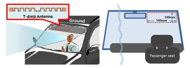
Figure 1: the available space of T-DMB antenna
