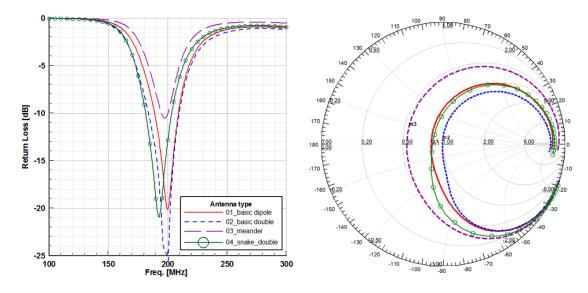
Figure 2: Impedance of Antennas.
