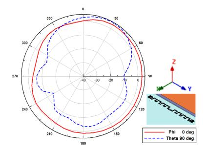
Figure 4: Radiation Pattern for the proposed antenna
