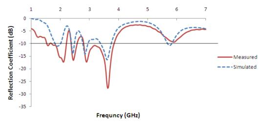
Figure 5: Measured and simulated reflection coefficient versus frequency (when  $L_8 = 13$ mm and  $L_9 = 11.5$ mm).
