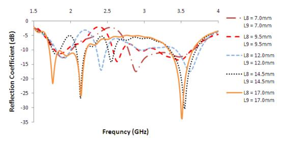
Figure 4: Simulated reflection coefficient versus frequency for various L<sub>8</sub> and L<sub>9</sub>.
