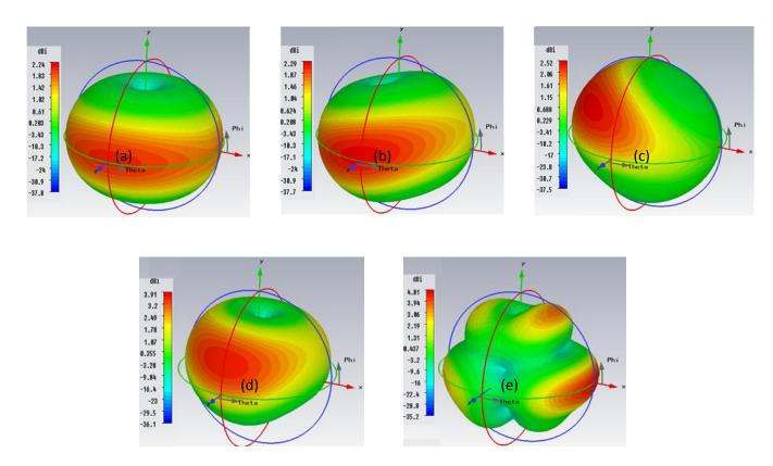
Figure 6: Simulated radiation pattern at (a) 1.9 GHz (b) 2.431 GHZ (c) 2.845GHz (d) 3.61 GHz and (e) 5.752GHz.
