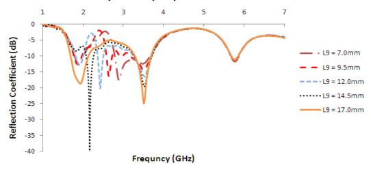
Figure 3: Simulated reflection coefficient versus frequency for various L<sub>9</sub>.
