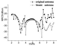
Fig.10. RCS comparison of the original patch antenna and the bionic antenna. ( $\theta = 60^\circ, \varphi = 90^\circ$ )
