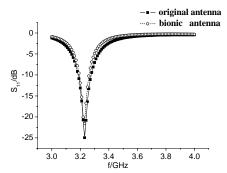
Fig.3. Simulated s11 comparison of the original patch antenna and the bionic antenna
