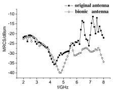
Fig.8. RCS comparison of the original patch antenna and the bionic antenna. ( $\theta = 60^{\circ}, \varphi = 45^{\circ}$ )
