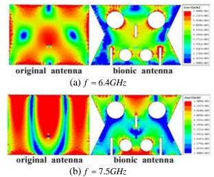
Fig.9. Current distributions of the original patch antenna and the bionic antenna ( $\theta = 60^\circ, \varphi = 45^\circ$ )
