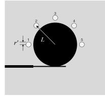
Figure 2. Geometry of the DGSs on the Circular Polarized Patch Antenna.
