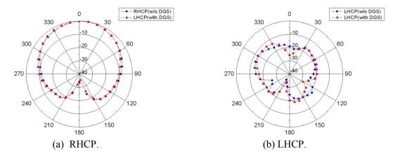
Figure 6. Radiation Patterns of the CP Antennas.
