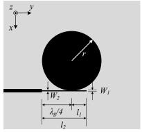
Figure 1. Configuration of the Tangential-Fed CP Antenna.
