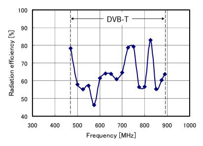
Figure 5: Measured radiation efficiency for installed antenna.
