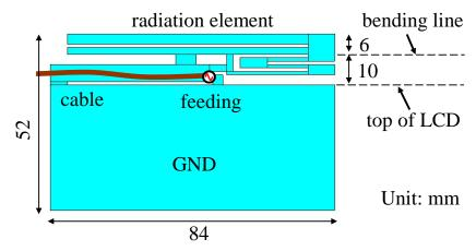
Figure 1: Antenna configuration in planar form.
