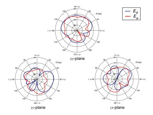
Figure 6: Measured radiation patterns at 700 MHz.
