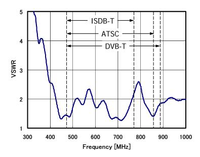
Figure 4: Measured input characteristics for installed antenna.
