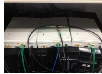
Figure 6: Implemented chaotic CDMA system on three USRPs, which is used for the experiments.
