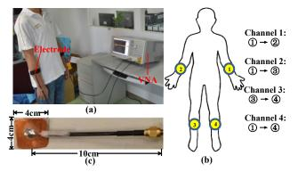
**Figure 1.** (a) Experimental scenario setup; (b)Measurement configuration, channel 1:left arm to right arm ;channel 2:left arm to left leg; channel 3:left leg to right leg; channel 4: left arm to right leg;(c) TX and RX signal electrode.
