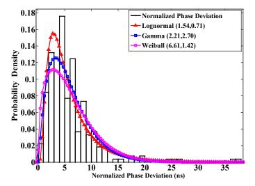
Figure 4. Empirical PDF of the normalized phase deviation for four channels and the fitting model
