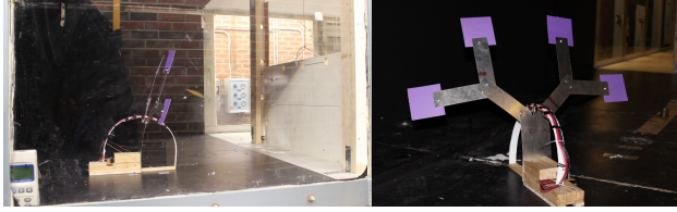
Figure 2: Pictures of the tree-like structure in wind tunnel. Left: the tree-like structure and flow barrier. Right: detail of the tree. The plastic semicircle contains coils with a circuit and LED for energy harvesting.
