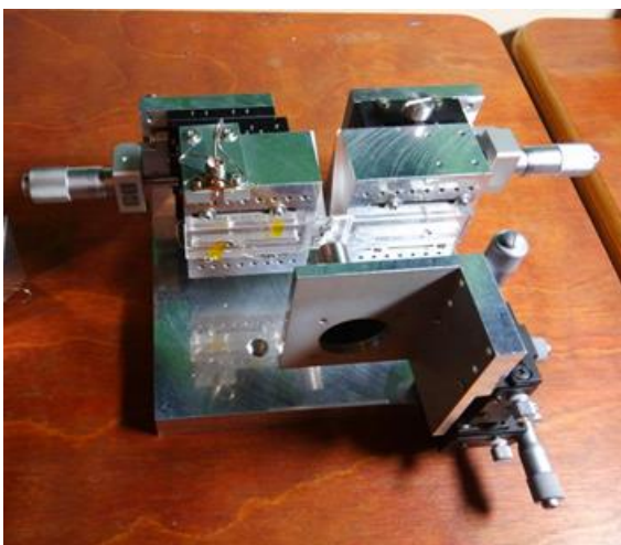
Fig.1 Metal V grooved waveguide with variable gap width.
