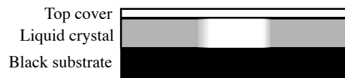
Figure 1: Schematic cross-sectional diagram of an opto-thermal bistable device based on nematic-isotropic phase transition of a liquid crystal. The light irradiated from top transmits through the liquid crystal layer and is absorbed in the black substrate to be converted to heat. The liquid crystal presents lower optical transmission due to optical scattering at low temperature in nematic phase (shown in gray), while it shows higher transmission at higher temperature in isotropic phase (shown in white). The wavefront, interface between gray and white area, can propagate laterally.
