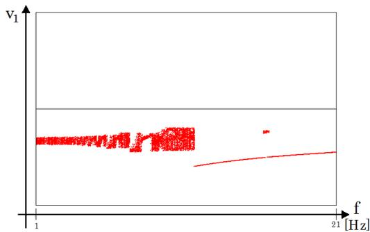
Figure 12: Bifurcation diagram for  $V_S = 1.2V$ .
