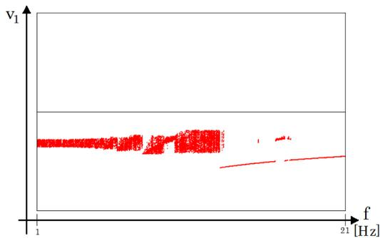
Figure 7: Bifurcation diagram for  $V_S = 1.0V$ .
