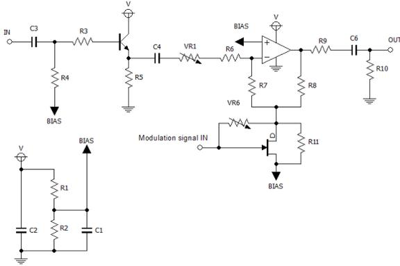
Figure 3: Amplitude-modulation circuit.
