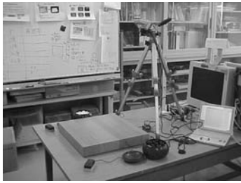
Figure 8: Prototype system for automatic generation of Go-record.
