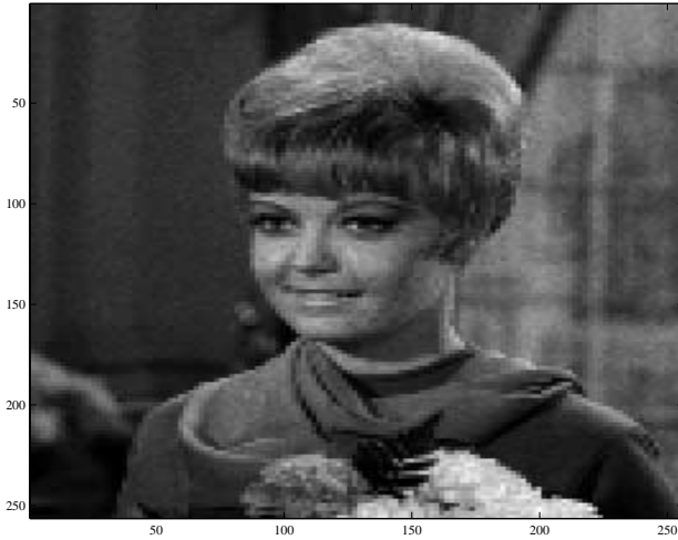
Interpolated Image (256 × 256) Using Zero-Order Hold
