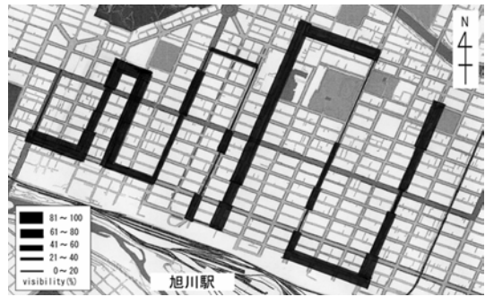
Fig. 6 Satellite visibility example for Asahikawa without Sat. D and TDD
