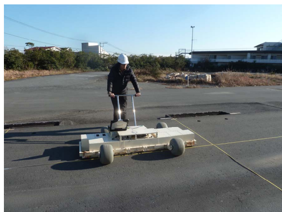
Fig.1 Multistatic GPR “Yakumo”.
