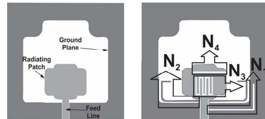
(a) UWB Antenna      (b) Quad band-notch antenna
