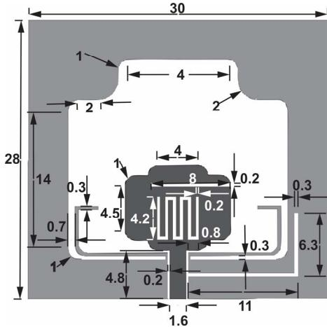
Fig. 2. Geometric structure of proposed quad band-notch antenna
