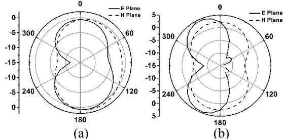
Fig. 5. H-Plane and E-Plane Radiation patterns at (a) 4 GHz (b) 8 GHz
