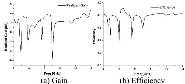
Fig. 4. Gain and efficiency of quad band-notch antenna
