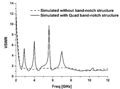
Fig. 3. Impedance match of proposed antenna with and without band-notch structure
