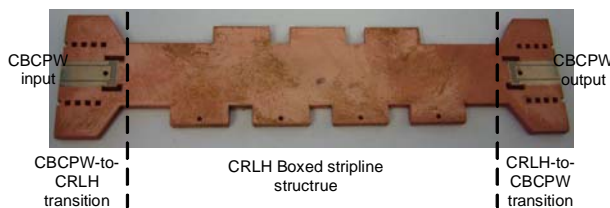
Fig.4 Prototype of a non-radiative CRLH boxed stripline structure.
