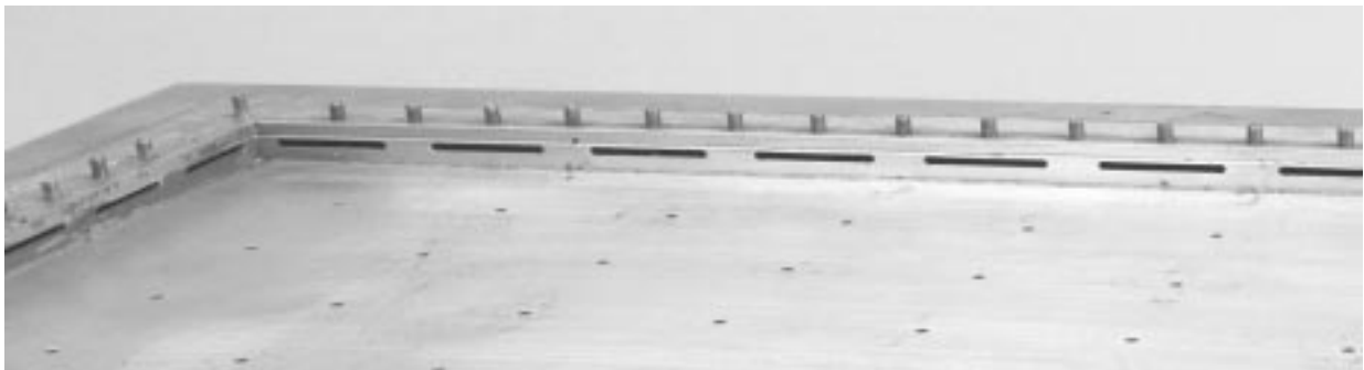
Figure 1. A view of some of the TE_{10,0} mode exciter slots in the narrow wall.
