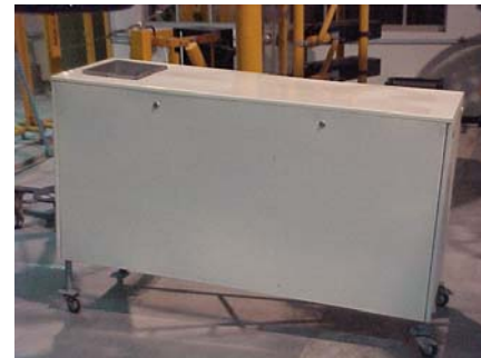
Fig. 9. Grass seed separation machine from broken milled rice by electric field technique.
