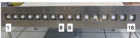
Fig. 4. 16-element array using cavity antenna. (Numbers in the picture indicate element No.)
