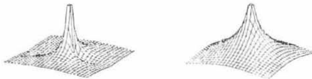
fig.3. Variation of normalized surface-wave amplitude for the TE1 mode components ( \Gamma_z -left, \Gamma_x -right) with radial distance in the vicinity of a x-directed electric dipole.
