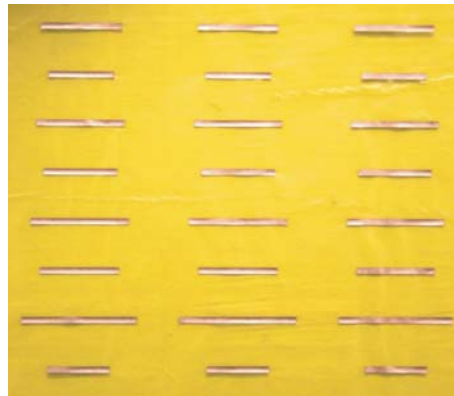
Fig. 9. Close-up photograph in the middle of fabricated reflectarray.
