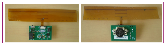
Fig. 5. Photograph of the realized power cord impulse sensing RFID tag
