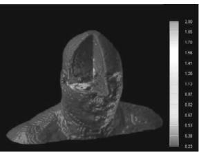
Fig. 4 Distribution of induced current density  $(J_{peak})$  in 1 mm Brooks model for cheek exposure
