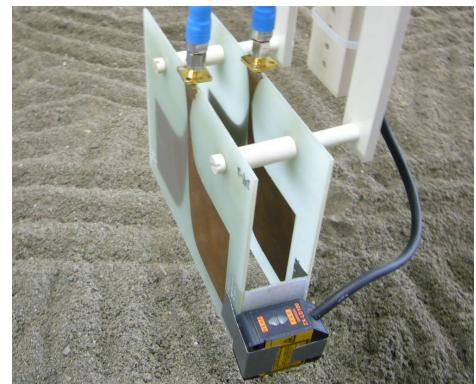
Figure2: Transmitting and receiving antennas (Vivaldi type).
