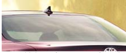
Figure 1: Present vehicle rooftop antenna for Telematics service
