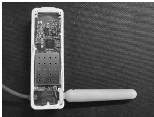
Figure 1: A monopole antenna used in WLAN Figure2: Multi-band nature of a monopole antenna
