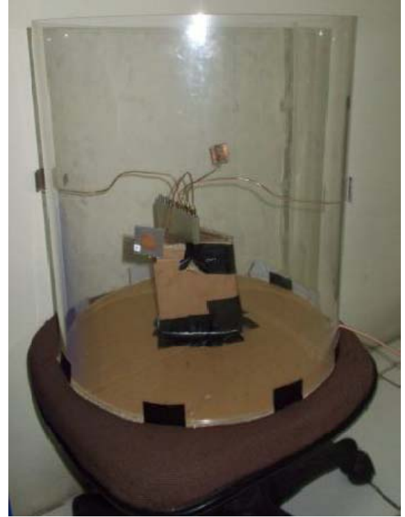
Fig. 3. The photograph of fabricated assembled antenna on the surface cylindrical fuselage
