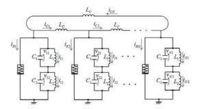
Figure 1: Ring of coupled simultaneous oscillators with two resonators.
