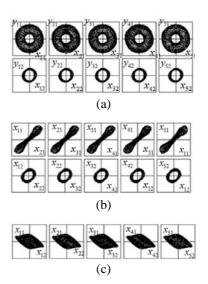
Figure 2: Typical example of obtained results from 5 coupled oscillators for  $\alpha_C = 0.8$ ,  $\alpha_L = 1.0$ ,  $\gamma = 0.3$ ,  $\varepsilon = 0.3$ , and  $\beta = 3.5$ . (a) Attractors observed at 10 resonators. Horizontal:  $x_{jk}$ . Vertical:  $y_{jk}$ . (b) Phase relationship between horizontally adjacent resonators. Horizontal:  $x_{j+1,k}$ . Vertical:  $x_{jk}$ . (c) Phase relationship between two resonators in each oscillator. Horizontal:  $x_{j2}$ . Vertical:  $x_{j1}$ .
