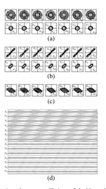
Figure 6: Asynchronous oscillations of double-mode and 7phase obtained from 7 coupled oscillators for  $\alpha_C = 0.8$ ,  $\alpha_L = 1.0$ ,  $\gamma = 0.3$ ,  $\varepsilon = 0.3$ , and  $\beta = 3.5$ . (a) Attractors observed at 14 resonators. (b) Phase relationship between horizontally adjacent resonators. (c) Phase relationship between two resonators in each oscillator. (d) Time waveforms of the voltages of 14 resonators
