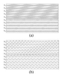
Figure 3: Time waveforms of the voltages of 10 resonators for  $\alpha_C = 0.8$ ,  $\alpha_L = 1.0$ ,  $\gamma = 0.3$ ,  $\varepsilon = 0.3$ , and  $\beta = 3.5$ .
