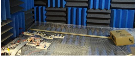
FIG. 6. Acoustic ranging system using solvable chaos installed in an anechoic test chamber.
