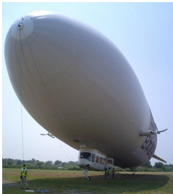
Figure 2. Ground handling of the Zeppelin NT airship at Honda Airport, Okegawa, Saitama Prefecture; note the relative size of the gondola.
