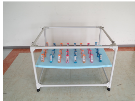
Figure 1: A frame and a board used for experiments on synchronization of 32 metronomes.
