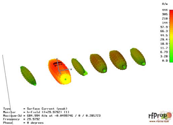
Fig. 11. Radiation of the Yagi-Uda (array) antenna – current distribution
