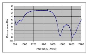
Fig. 5: Measured input return loss
