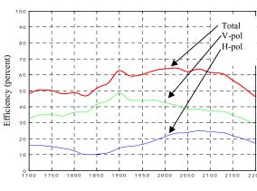
Fig. 4: Measured terminal efficiency of the handset in the low bands (above) and high bands (below).
