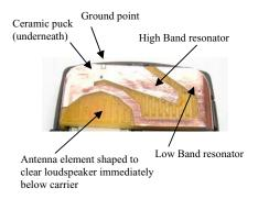
Fig. 3: View showing topology of the antenna
