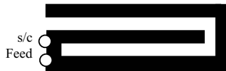
Fig. 2: Simplified antenna layout from which the shape shown in Fig.1 was derived.
