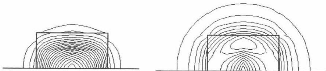
Fig. 3 : The power distribution for the first and second modes in the image waveguide at k_0c=2.0
